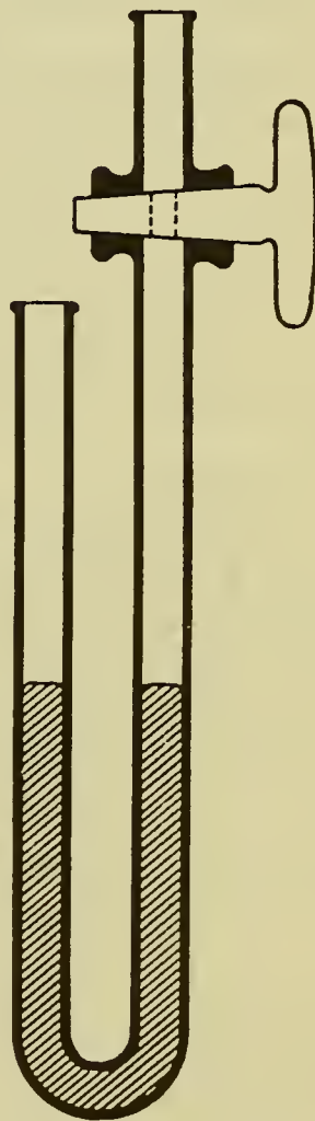
FIG. 11. Apparatus controlling the density of air in the cabin
