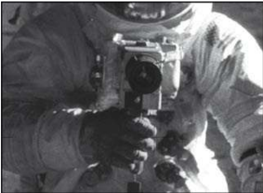
6. Close up lunar camera on chest bracket.
