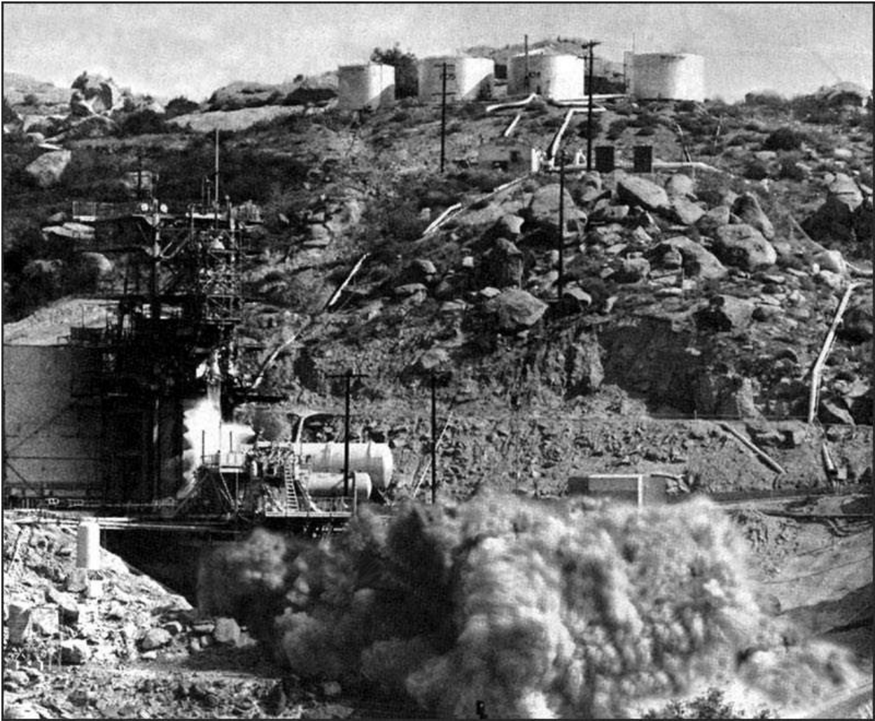
42. Hypergolic tests in the Simi Hills, California which produced thick, dense, opaque, dark red smoke. W KAYSING
