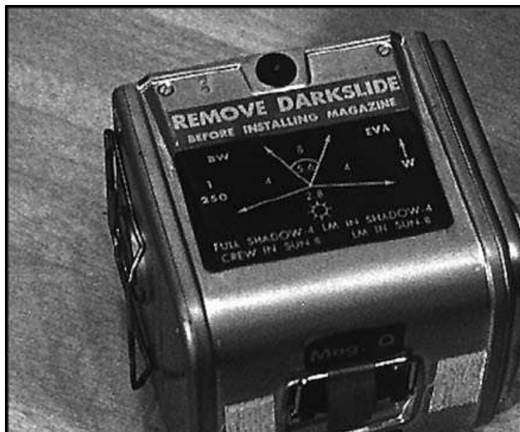
8. Exposure guide on camera magazine. AULIS
